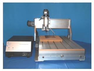
StepTwo is the "entry level" in the field of rapid prototyping of PCBs and in small batches productions.
